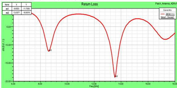
Figure (2) Return loss Vs Frequency
